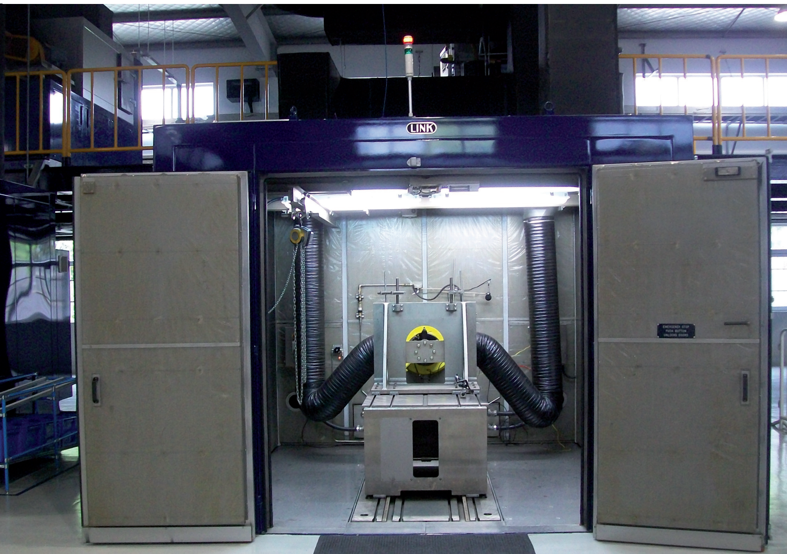
Installed new inertia brake dynamometer: View into the walk-in NVH test arrangement
