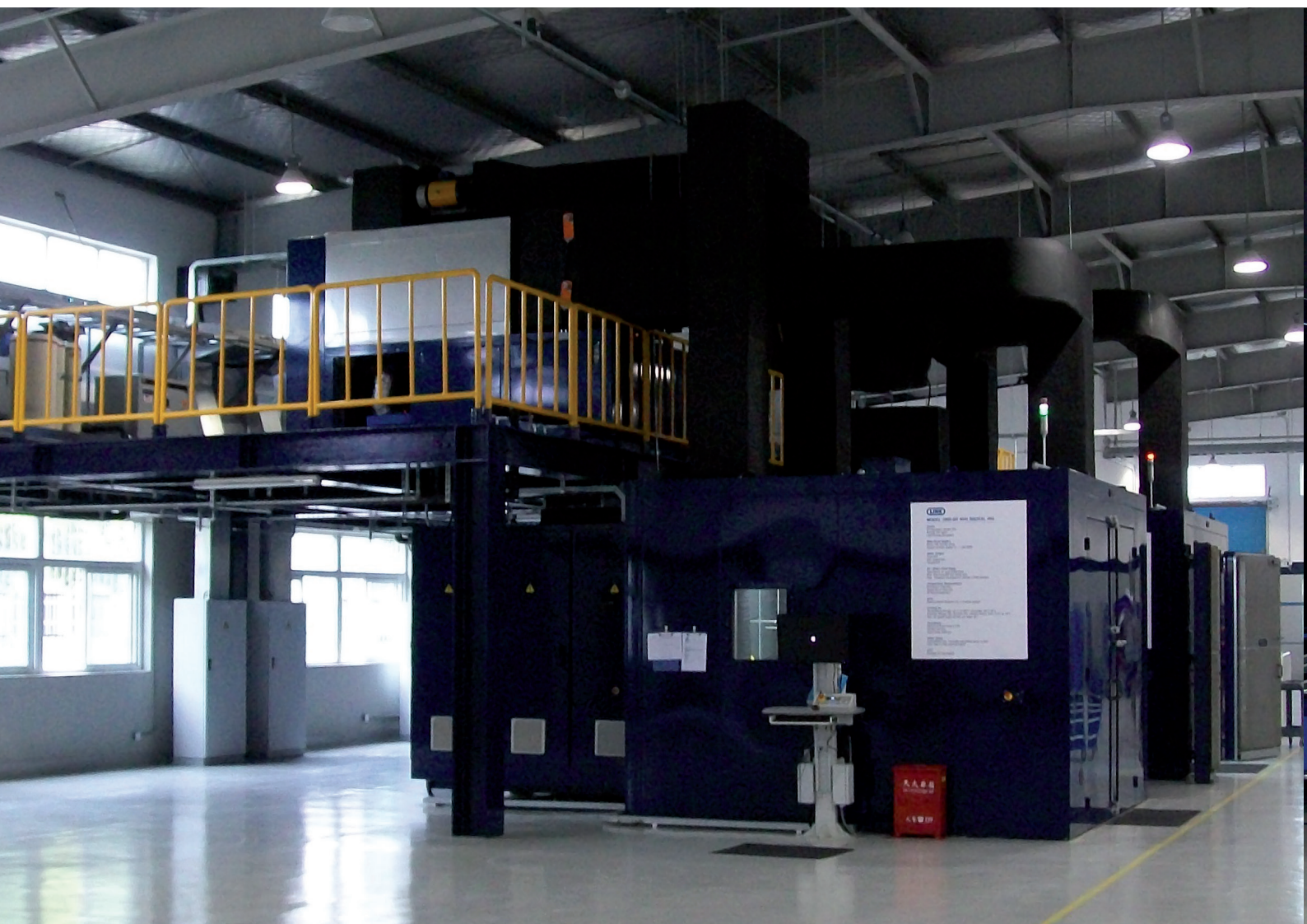
Installed new inertia brake dynamometer: Top left with environmental conditioning unit
